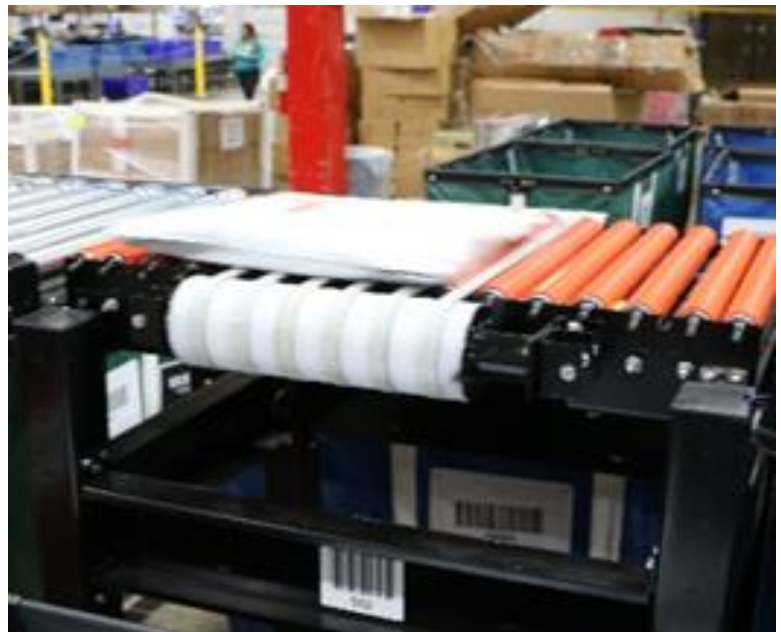
Sideview of Z1 eSorter in action: Lifting, and positively sorting a soft sided poly bag, while briefly pausing the forward rollers to eliminate any opposing force on the Poly Bag...
